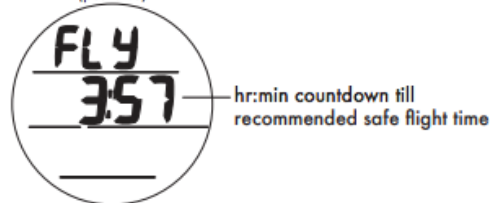
GAUGE STANDBY MODE (post dive)
