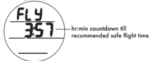
GAUGE STANDBY MODE (post dive)
