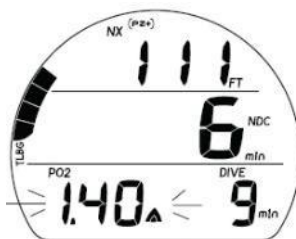
Fig. 57 - PO2 ALARM (until < Set Point)
