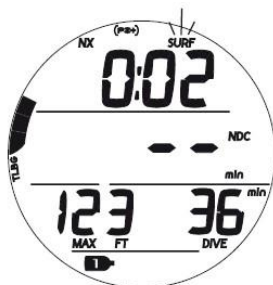
Fig. 74 - NO DECO MAIN (during < 10 min on surface)
