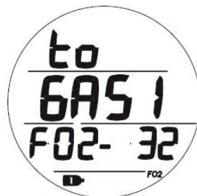
Fig. 98 - GAS 1 SWITCH PREVIEW
